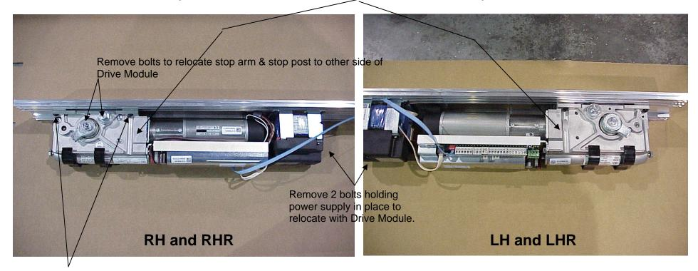
Remove 4 bolts to remove Drive Module to turn it over and mount at other end of back plate for hand change. Locate pinion on center at 5 1/2"
